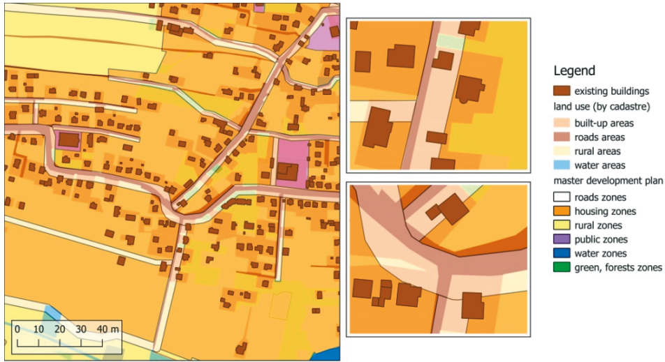
Figure 7: Verification of the local development plan arrangements with official land use map.
