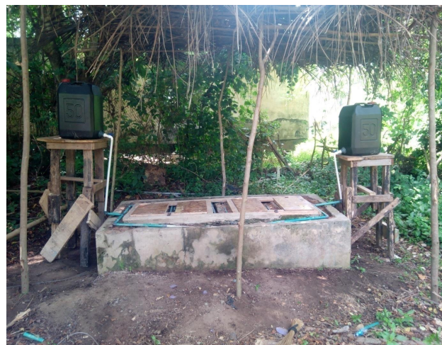
Fig. 1. Evaporative cooling chamber with water reservoir
