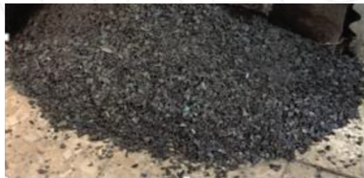
Figure 1. Polyethylene waste after cutting and grinding [10].
