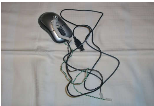
Figure 9 The picture shows an optical mouse that has been modified so that it can be used to measure the interval of the time
