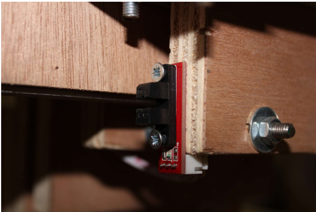
Figure 12: End-stop positioning on Y axis
