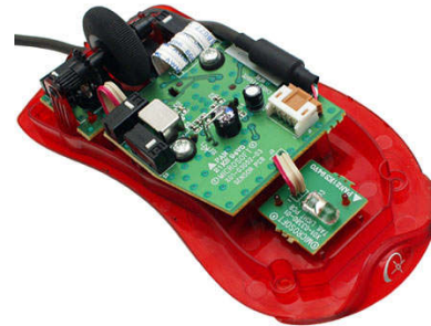
Figure 4 Interior of an optical mouse (ref.1)
