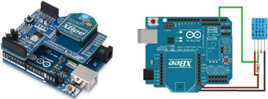
Figure 4 Hardware layout of Coordinator and Router device
