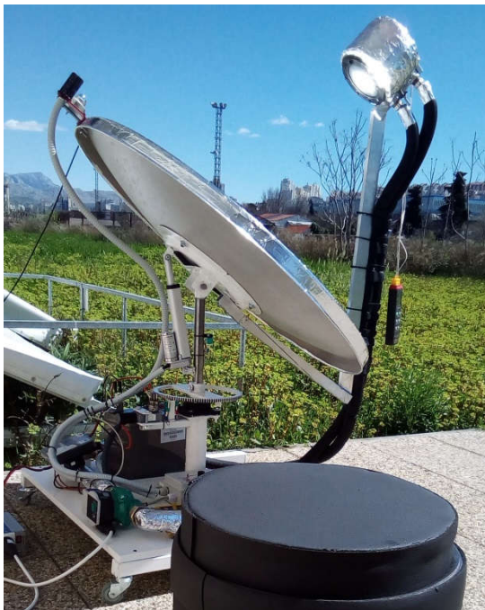
Figure 10 Parabolic dish concentrator in operation
