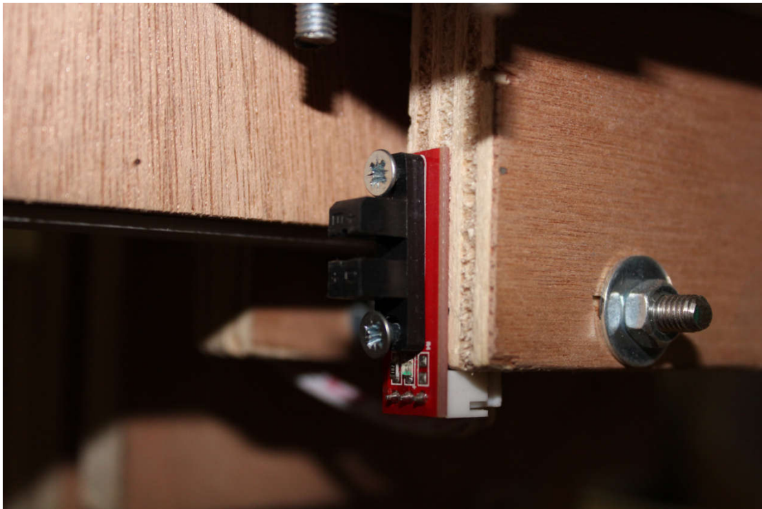
Figure 12: End-stop positioning on Y axis
