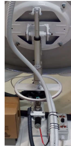
Figure 5 View of dual axis mechanism
