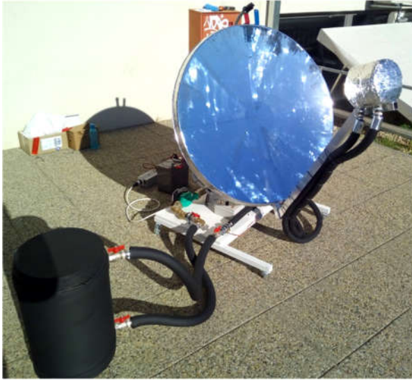
Figure 2 View of parabolic dish concentrator
