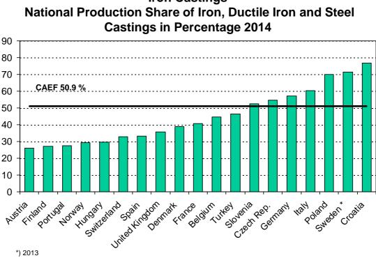
**Ductile Iron Castings** National Production Share of Iron, Ductile Iron and Steel **Castings in Percentage 2014**
