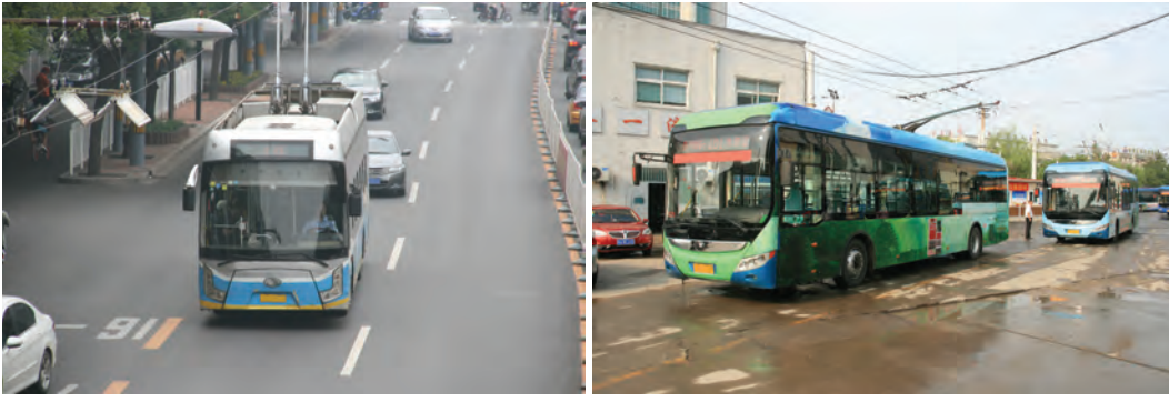
12-meter trolleybuses in the cities of Beijing and Jinan, People's Republic of China. Source: Asian Development Bank.
