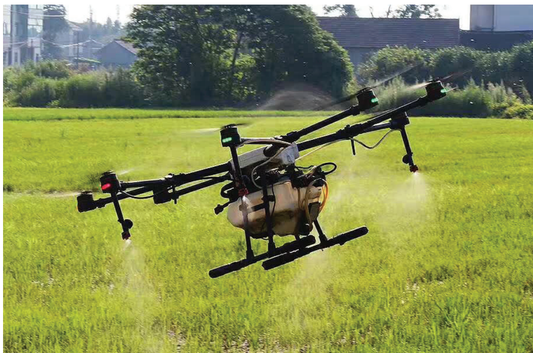
Unmanned aerial vehicle (UAV). An important application of the Internet of Things for modern agriculture is the use of UAV for pesticide spraying (photo by Haiping Jiang).
