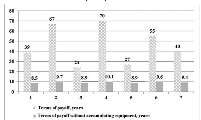
Figure 5: Terms of payoff of various options for the layout of a solar power plant
