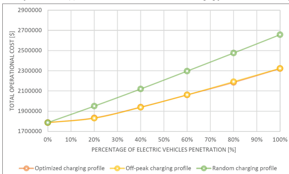
Figure 7: Total operational cost ($) of the stochastic model under different charging profiles for various EVs penetration
