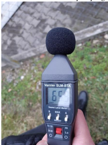
Figure 9: Noise meter at the pumping station
