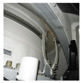
Figure 3.2 Lightning current transfer unit, LCTU
