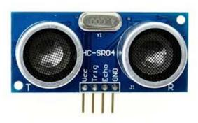
Figure 5 Ultrasonic Sensor HC - SR04
