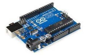
Figure 4 Arduino UNO microcontroller plate
