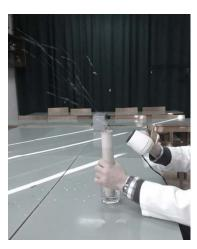
**Figure 7** An example of a simple experiment – "Beroulli's principle -Chimney". During the blowing of the hairdryer.
