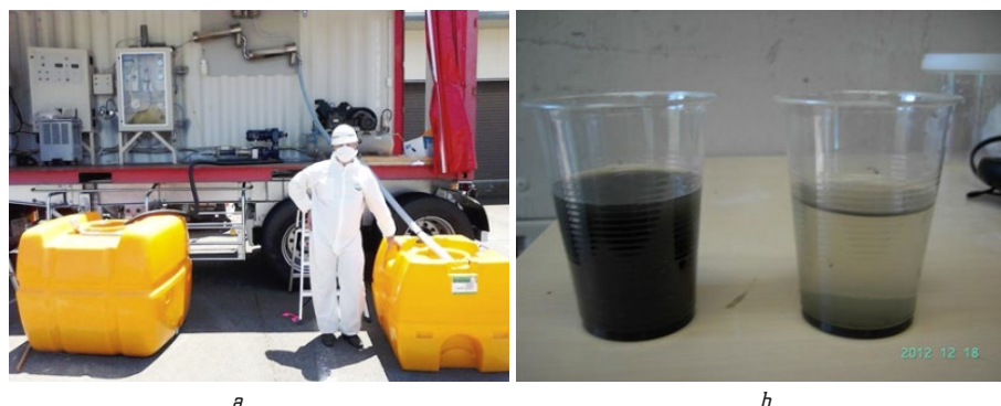
Fig. 2. Plasma treatment of contaminated soil in Fukushima Prefecture: a – mobile plasma-chemical setup; b – water before and after plasma treatment
