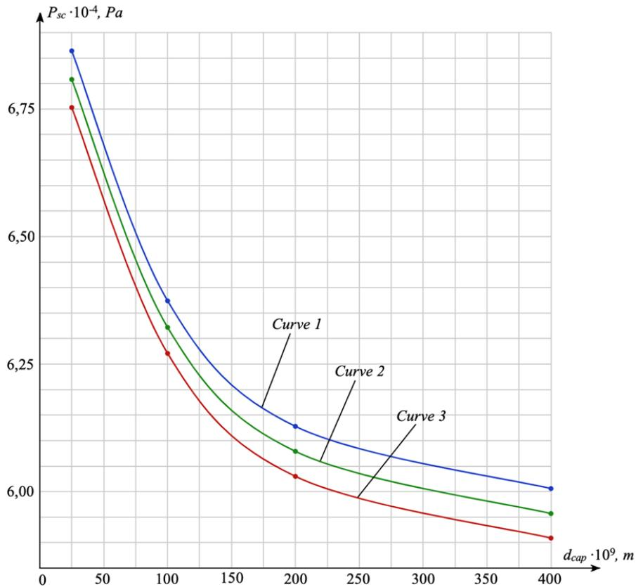
**Fig. 3.** Dependence of sound capillary pressure  $P_{sc}$ , Pa on capillary diameter  $d_{cap}$ , m for 70 % ethanol solution as an extractant: Curve 1 – at a temperature of 20 °C; Curve 2 – at a temperature of 30 °C; Curve 3 – at a temperature of 40 °C
