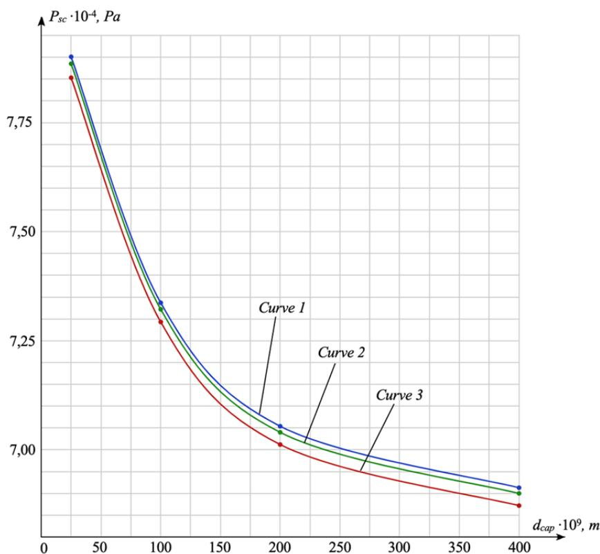
**Fig. 1.** Dependence of sound capillary pressure  $P_{sc}$ , Pa on capillary diameter  $d_{cap}$ , m for water as an extractant: Curve 1 – at a temperature of  $20\text{ }^{\circ}\text{C}$ ; Curve 2 – at a temperature of  $30\text{ }^{\circ}\text{C}$ ; Curve 3 – at a temperature of  $40\text{ }^{\circ}\text{C}$
