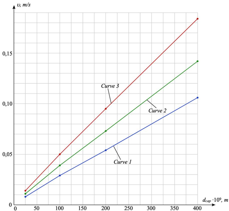
**Fig. 6.** Dependence of the penetration rate  $v$ , m/s of the extractant into the capillaries on the diameter of the capillaries  $d_{cap}$ , m for 70 % ethanol solution: Curve 1 – at a temperature of 20 °C; Curve 2 – at a temperature of 30 °C; Curve 3 – at a temperature of 40 °C
