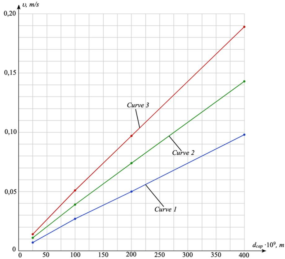
**Fig. 5.** Dependence of the penetration rate  $v$ , m/s of the extractant into the capillaries on the diameter of the capillaries  $d_{cap}$ , m for 40 % ethanol solution: Curve 1 – at a temperature of 20 °C; Curve 2 – at a temperature of 30 °C; Curve 3 – at a temperature of 40 °C
