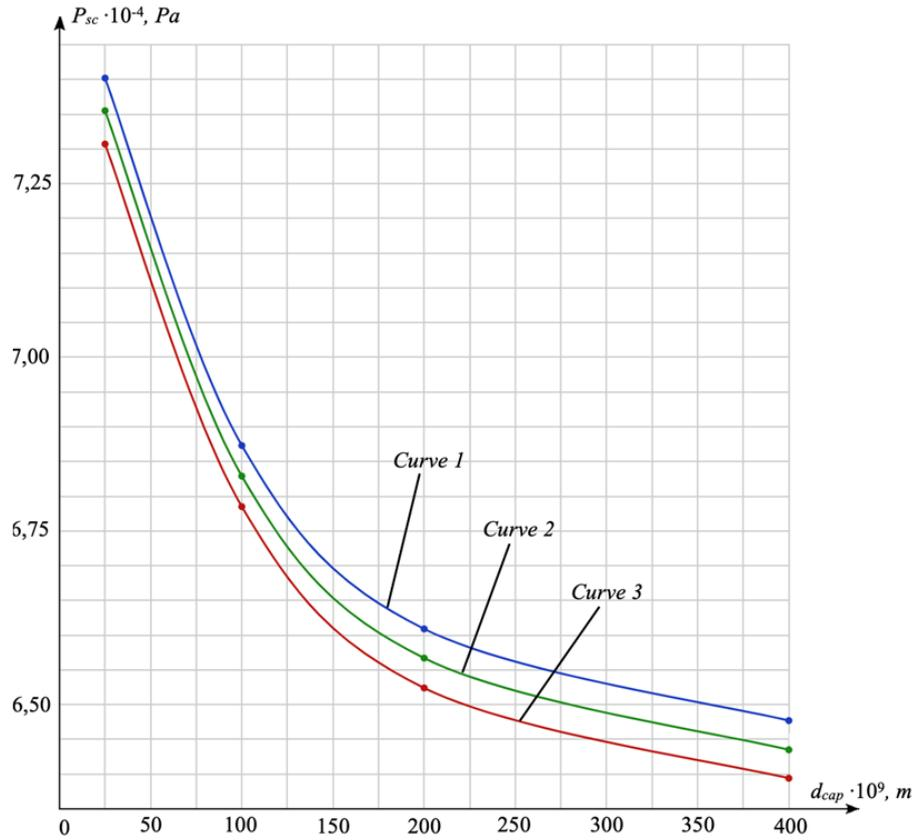
**Fig. 2.** Dependence of sound capillary pressure  $P_{sc}$ , Pa on capillary diameter  $d_{cap}$ , m for 40 % ethanol solution as an extractant: Curve 1 – at a temperature of 20 °C; Curve 2 – at a temperature of 30 °C; Curve 3 – at a temperature of 40 °C
