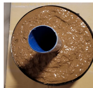
Fig. 5. Filling the container with water-saturated loam
