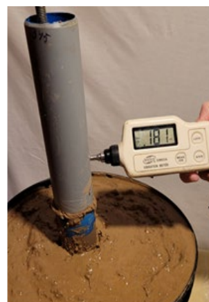
Fig. 6. Photo of a metal rod with a plunger and a manual contact vibrometer GM63A
