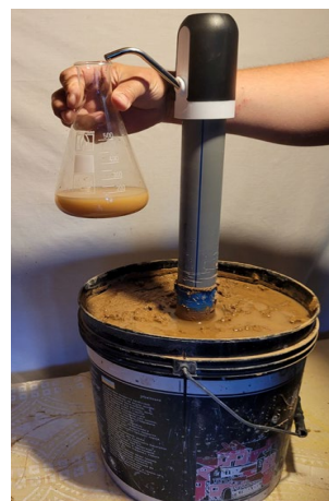
Fig. 7. Determination of fluid flow to the well after 12 hours of rest
