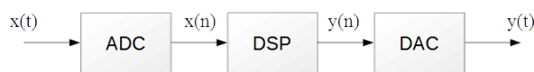
Fig. 1. General structure of the DSP system: ADC – analog-to-digital converter; DSP – digital signal processor; DAC – digital-to-analog converter
