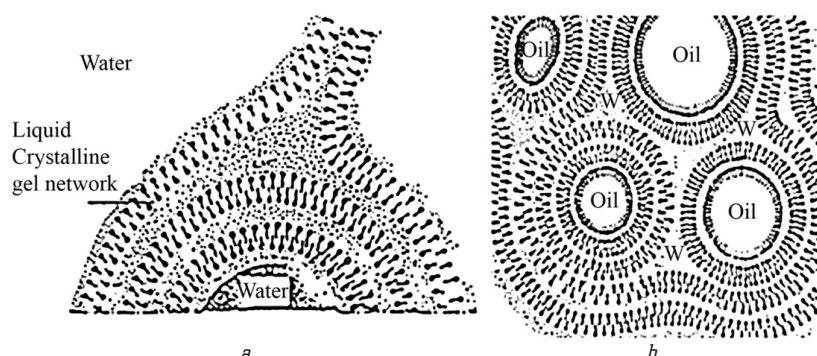
Fig. 1. Schematic representation of a lamellar liquid crystal emulsion [8]: a – with the encapsulation of the liquid phase (water); b – with the encapsulation of the fat phase (oil)
