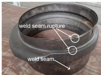
Fig. 8. The appearance of the weld seam rupture after the explosive forming
