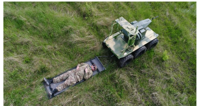
Fig. 3. Example of the evacuation of a simulated wounded person with the RSVK-M3 combat vehicle
