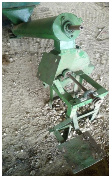
Fig. 2. Constructed Palm Nut Cracking Units
