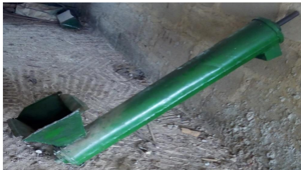
Fig. 4. Conveyor with Hopper
