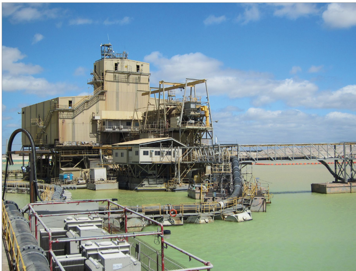
Figure 15: Floating wet mill at Cooljarloo. Photo BGR.
