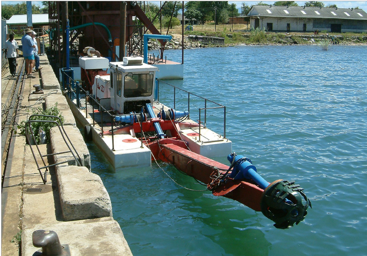
Figure 21: Small suction dredge and pilot wet mill behind for trial mining at Chipoka Bay in 2006.
