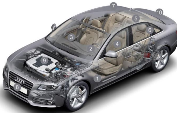
Figure 3: Car parts made of natural fibre composites
