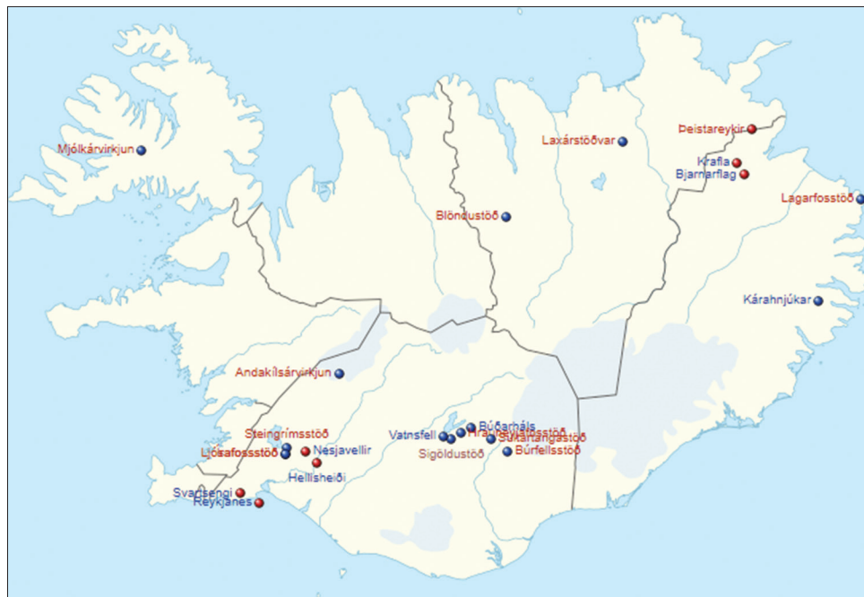
Figure 1: Map of energy plants in Iceland (blue – geothermal energy plants, red – hydro energy plants)
