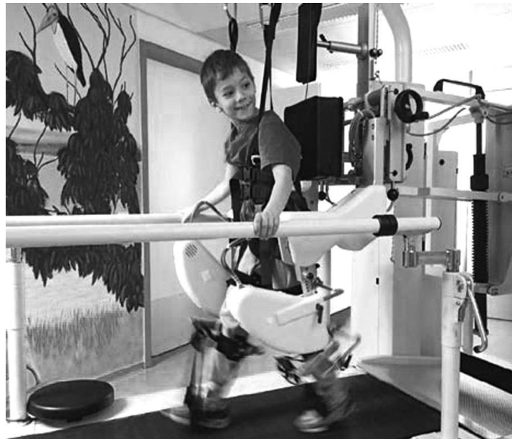
Figure 1: Robot Lokomat for strengthening the lower extremities
