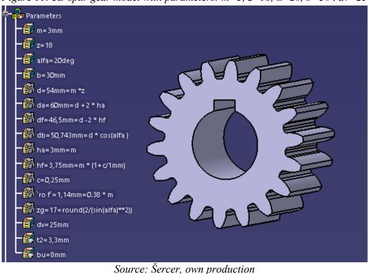
Figure 11: 3D spur gear model with parameters: m=3, z=18,  $\alpha=20$ , b=30 i dv=25
