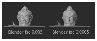
Figure 11 Blender Decimate modifier with two last factors
