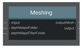
Figure 3 Meshing node creates a mesh from Structure from Motion (SfM) data
