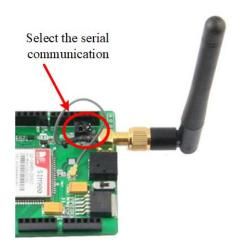
Figure 5 Selecting the serial communication
