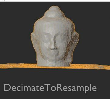
Figure 16 Final result after serial connection of MeshDecimate and MeshResampling nodes
