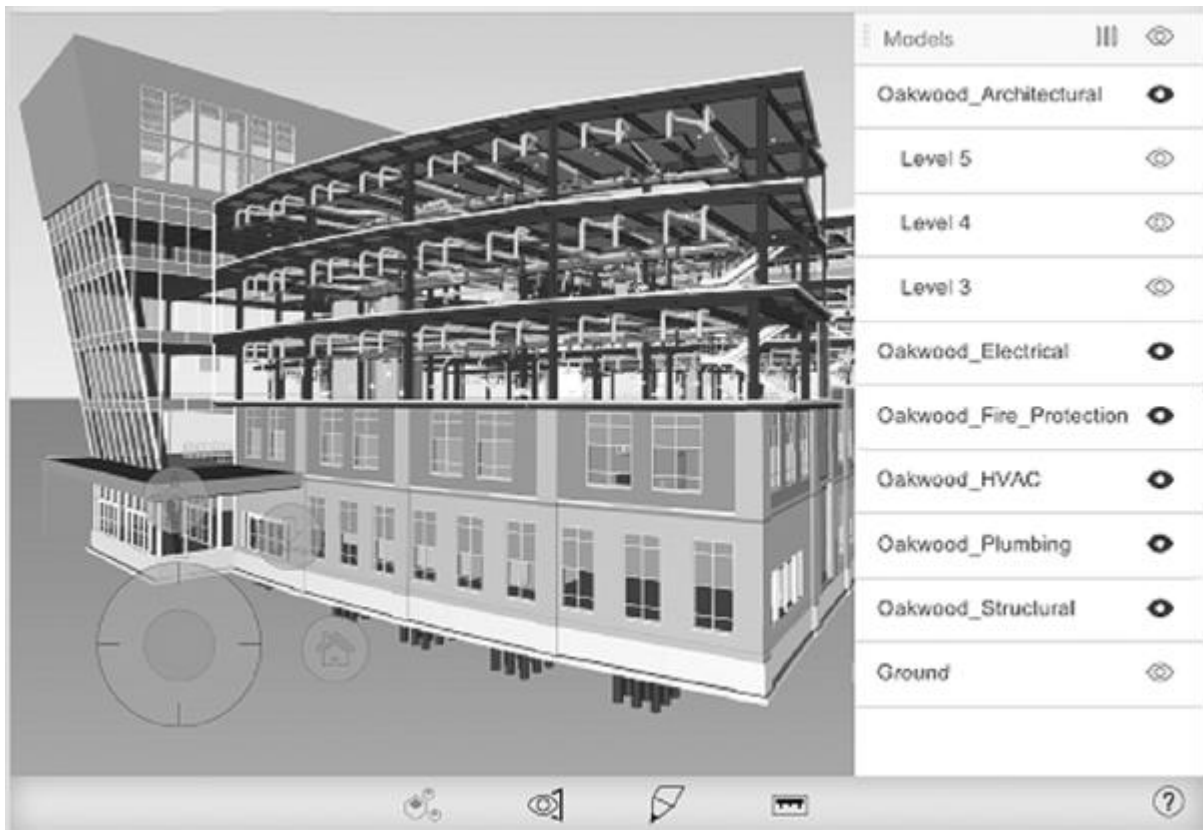
Figure 4: 3D-model of a building constructed using BIM
