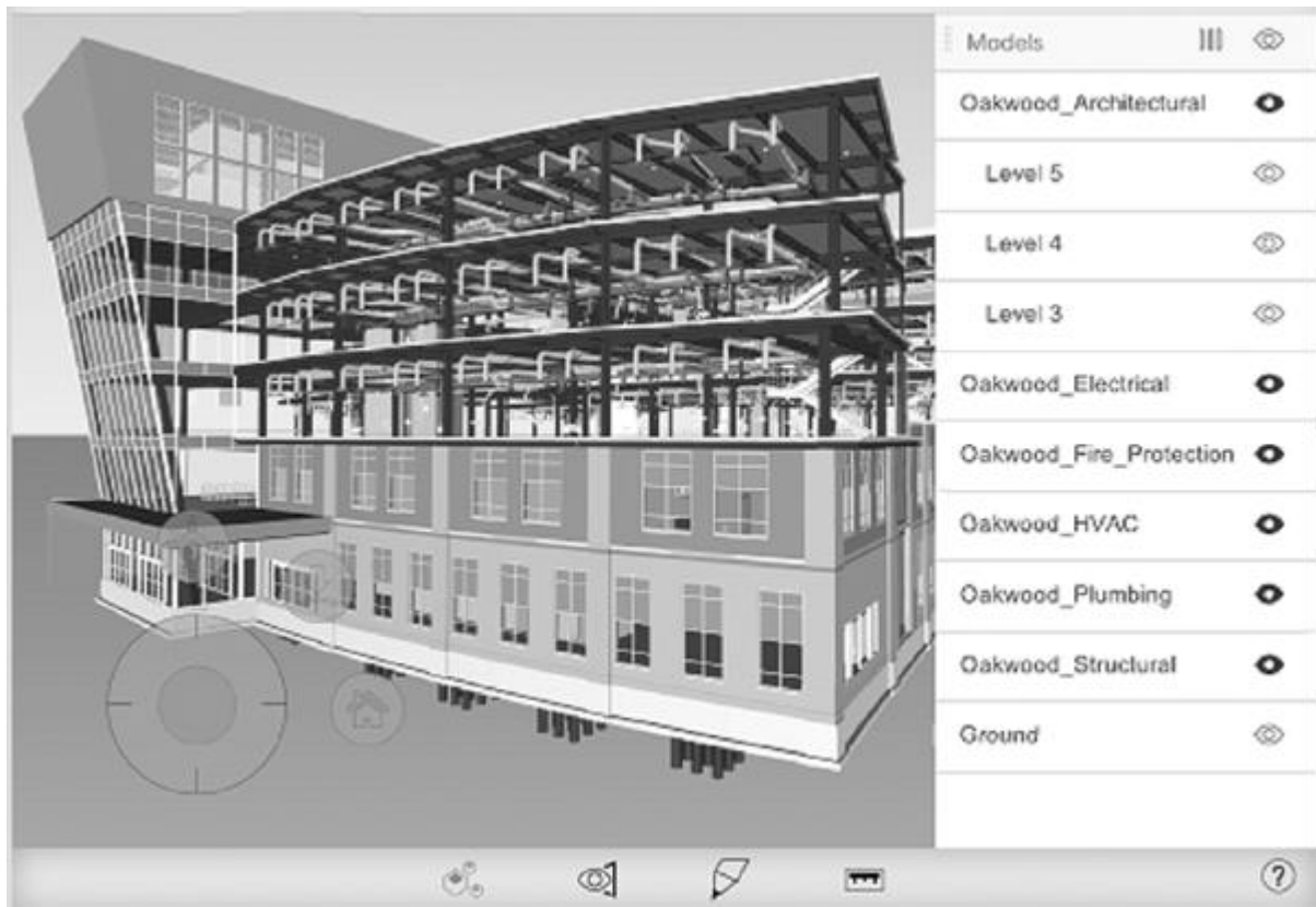
Figure 4: 3D-model of a building constructed using BIM
