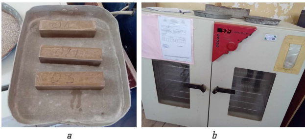
Fig. 6. Accelerated humidification-drying aging cycle: a – specimens; b – oven
