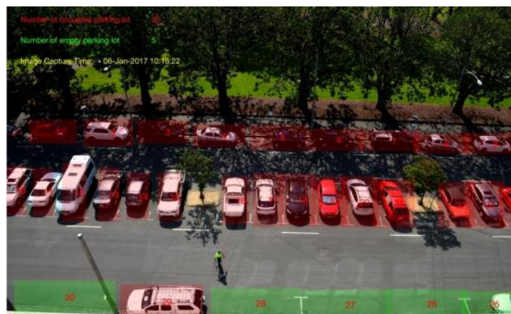
Figure 3: Smart parking system based on image processing (Acharya, Yan, Khoshelham, 2018, pg. 38)
