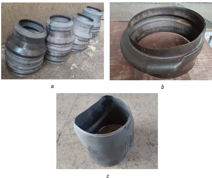
Fig. 13. Samples of parts, obtained by explosive forming using an intelligent process optimization system: a – series of «Stator» parts; b – «Volute» («Cochlea») part; c – «Housing» part
