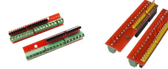
Figure 14 "Proto Screw" shield
