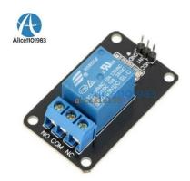
Figure 5 Relay board
