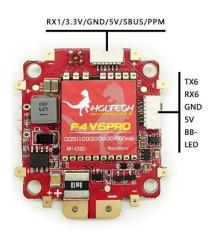
Figure 9 HGLRC F4 V6 PRO top view
