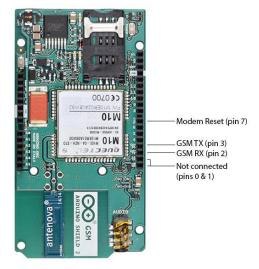
Figure 3 GSM shield
