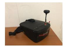
Figure 12 FPV goggles Eachine EV800
