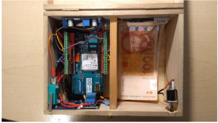
Figure 15 Fully operating deposit box
