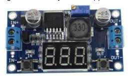
Figure 11 Power supply based on LM2596
