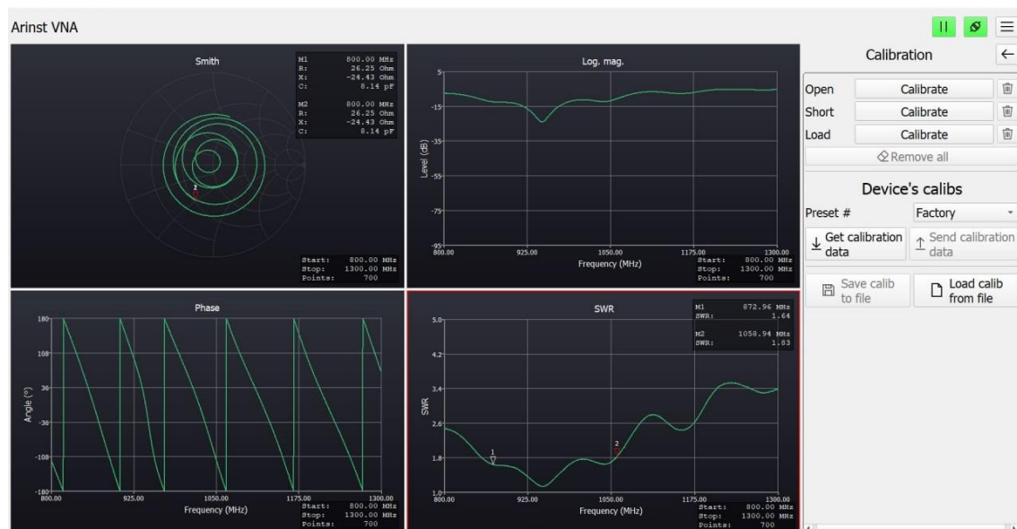
Fig. 9. Results of experimental studies of a flexible bracelet antenna when filling a Teflon glass with mineral water
